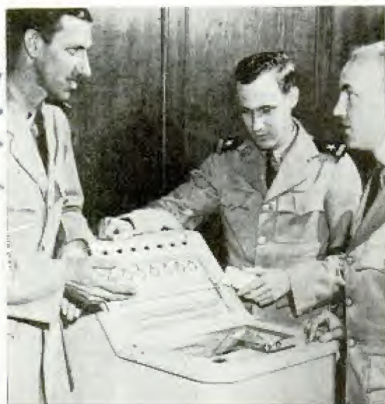
Push-button quizzer for naval aviation cadets tests speed and accuracy in identifying ships and aircraft
